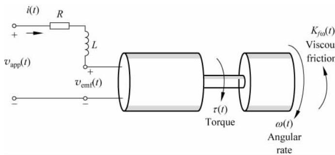
Fig. 3-8-1 A simple model of the DC motor
