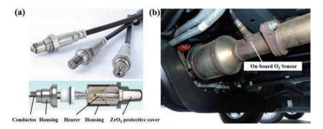
Fig. 1.4 a Structural diagram of on-board oxygen sensor; b Working principle of oxygen sensor in automobile exhaust system
