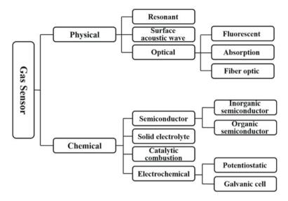
Fig. 1.3 Classification of gas sensors
