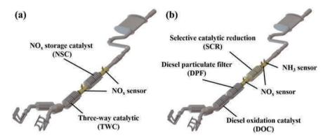
Fig. 1.5 a Lean combustion technology of gasoline vehicle exhaust purification system; b Diesel vehicle exhaust purification system
